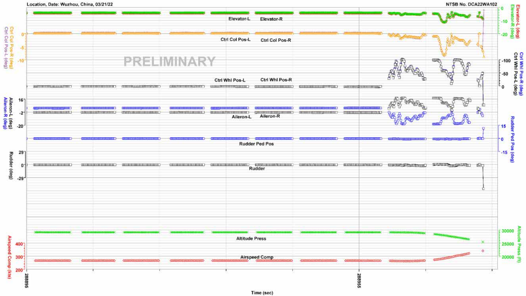
Figure 12. Flight control and input positions for final 90 seconds of recording.
