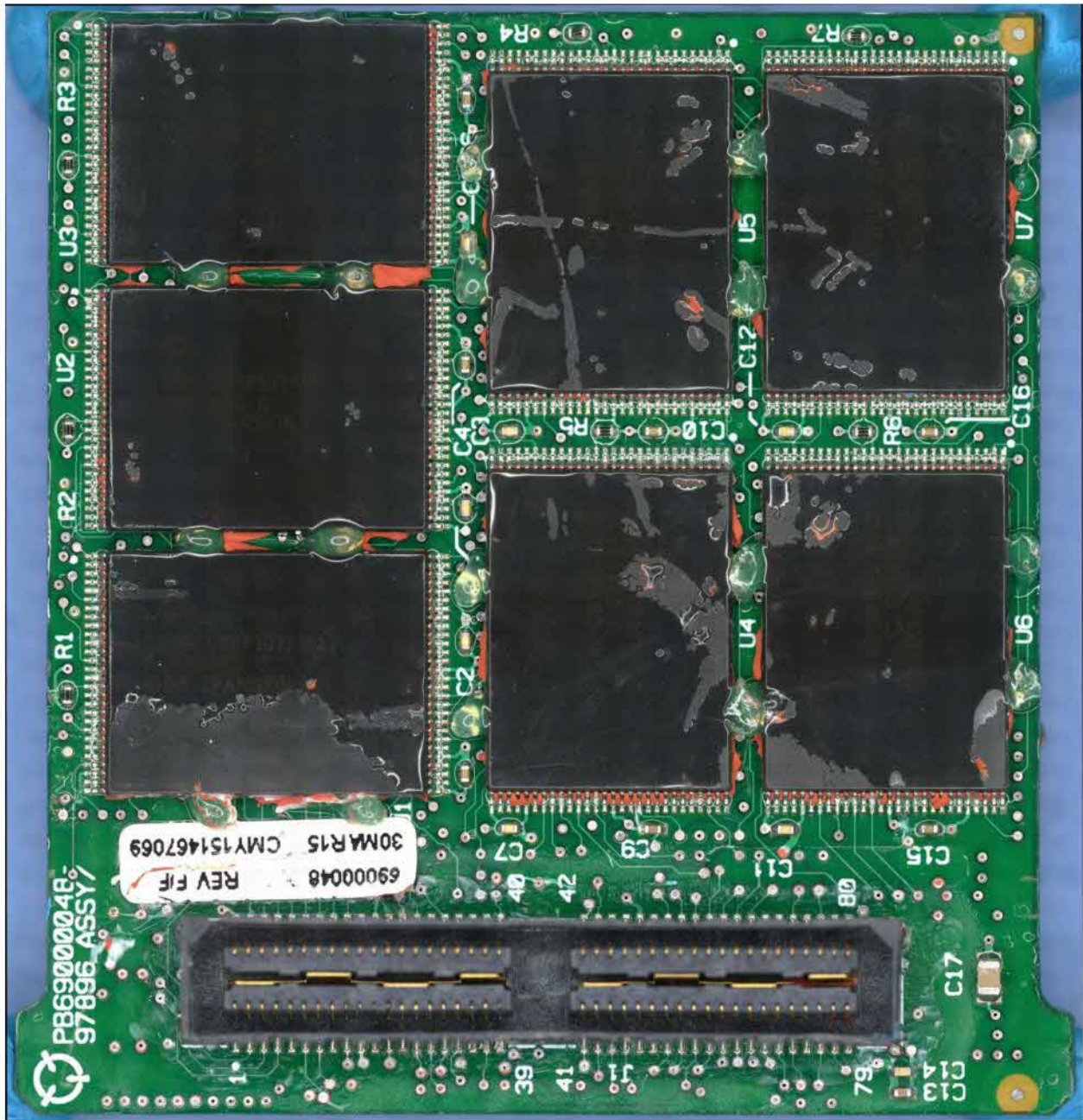
Figure 1. CVR memory module board, connector side.
